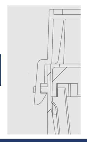
A positive snap lock system to lock the tip box perfectly.
