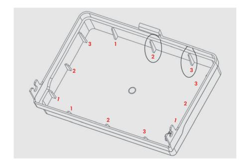
12 no's (3-3-3-3) of ribs has been incorporated all around tip box Bottom & Lid respectively to enhance strength
