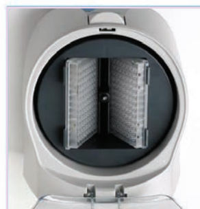
Before & after centrifugation (angled position)
